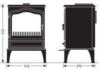
Distance from centre of flue to back of stove 145mm. Distance from hearth to centre of flue 390mm.
