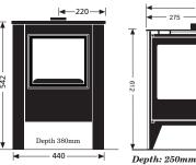
Distance from centre of flue to back of stove 140mm. Distance from hearth to centre of flue 415mm (585)
