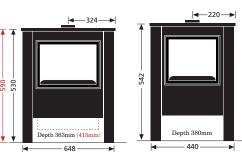
Distance from centre of flue to back of stove 145mm (135mm). Distance from hearth to centre of flue  $405 \mathrm{mm}$ (453mm). \*225 ONLY
